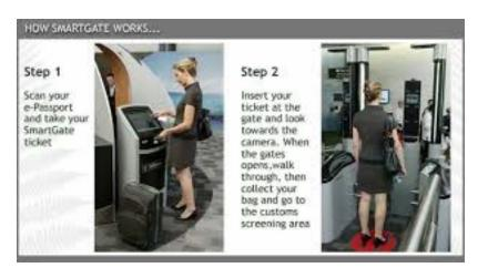
for the kiosk and ticket. The solution uses "face-on- the-fly" technology. The current installation is 8 facial recognition departure egates, 14 arrival e-gates, 17 departure kiosks, 36 arrival kiosks. A three-dimensional facial image of a user's face is taken as the individual approaches the gate and then compares it to the image stored in a presented e-passport. The individual barely has to slow down
