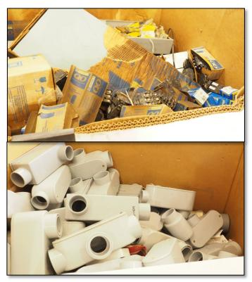
Figure 5: New breakers (top) and conduit body joints w/cover (bottom) slated for destruction/disposal
