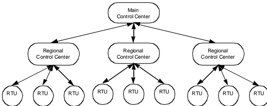
They communicate externally in a variety of ways. They use leased phone lines, dial-up phone lines, and LAN/WAN communications. These are usually provided by a local telecom. In addition, devices are commonly connected to the remote ends by additional communication methods, including hard wire contacts, radio, satellite, and microwave. Wireless technologies are being used more and more for connections to sensors.
